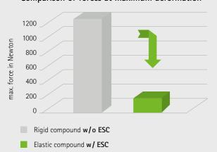
Case study: 48 mm sandwich panel, 3 mm aluminum sheeting outside / 43.5 mm foam core w/o ESC / 1.5 mm aluminum sheeting inside
